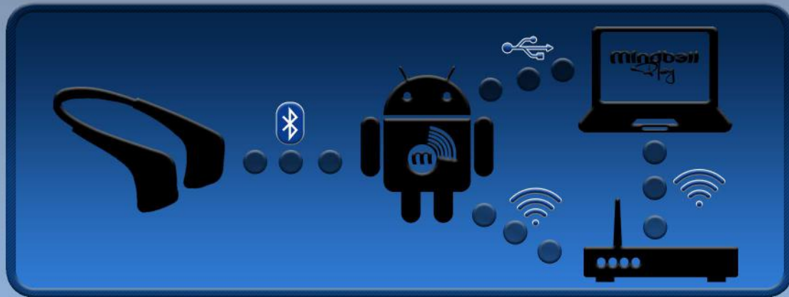
How the bridge setup needs to be configured. Note that the USB connection between the Android device and the PC isn't necessary if they're already on the same wifi network.
